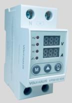
Voltage monitoring relay VPS8 series is designed to protect household equipment from high or low mains voltage, as well as overcurrent (if applicable), with an automatic recovery function after operation. They are used in the construction of input and distribution electrical panels in apartments, country houses, office and industrial facilities. They are used in AC electrical circuits with a frequency of 50/60 Hz, rated voltage 220 V.
